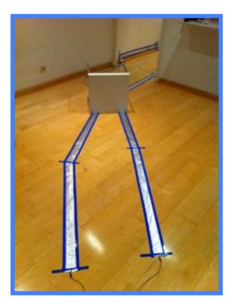
Note the wires on each path that are connected to ground and any key in the Makey Makey.
