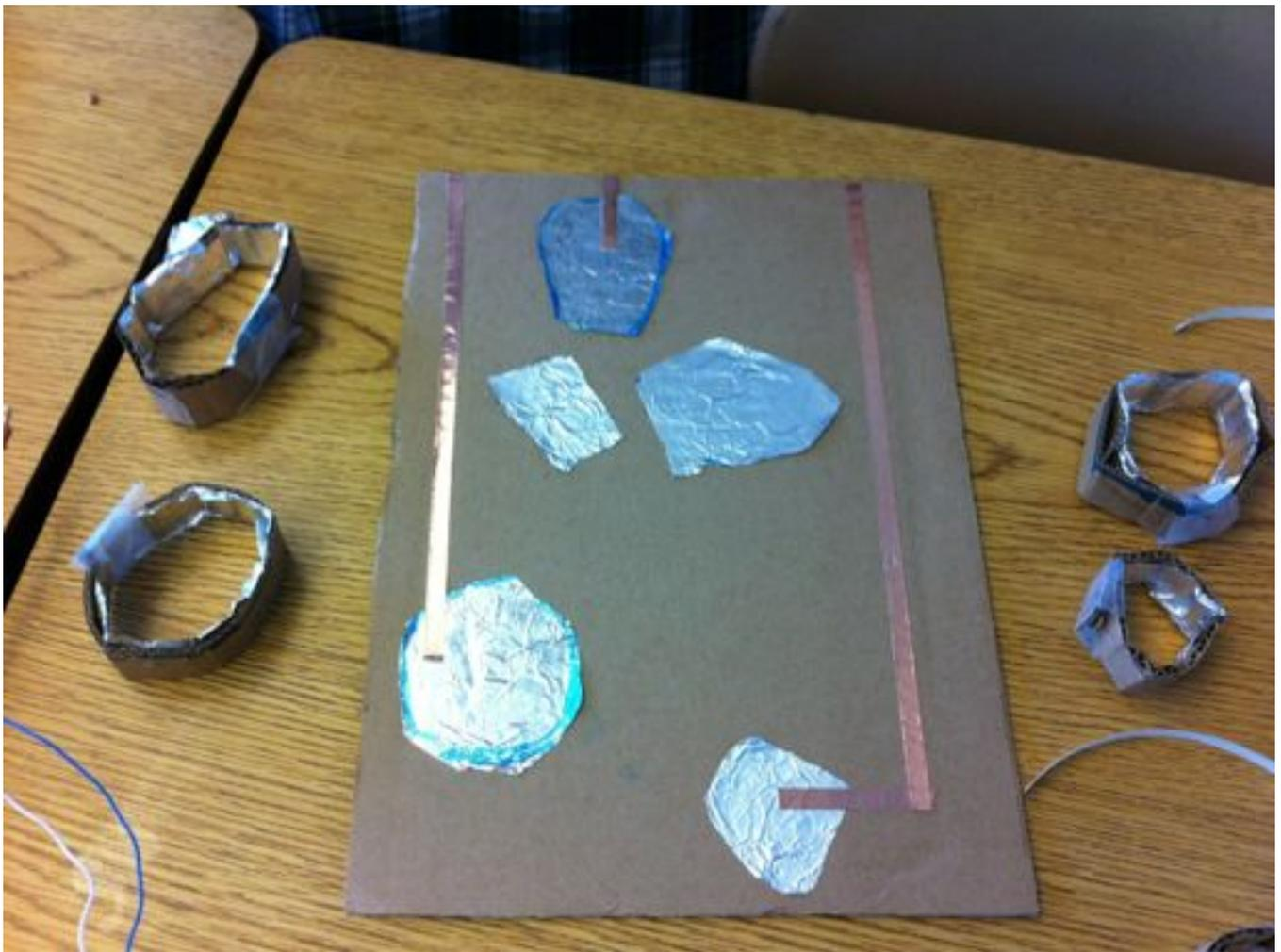
Measure as many strips of cardboard as you have holes in your box. You want the strips of cardboard to be equal in width so the motherboard sits flat against the inside top of the box. Use a glue stick to glue aluminum foil to these cardboard strips. Bend the cardboard into the shape of the hole you traced on the motherboard. Use a hot glue gun and hot glue to attach the "cups" to your motherboard.
